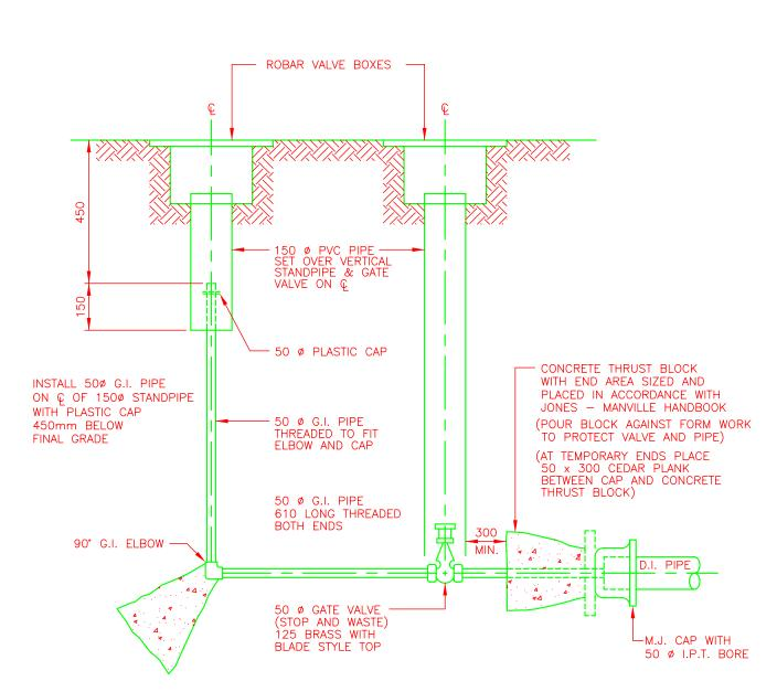
NOTE: VALVE AND PIPE ASSEMBLY MAY COME OFF THE SIDE OF THE PIPE AT A 90° ANGLE TO ALLOW FOR A STANDARD THRUST BLOCK AT THE END OF THE CAPPED MAIN. THE PIPE SHOULD BE THREADED TO THE MAIN WITHIN 500mm FROM THE CAPPED END.
